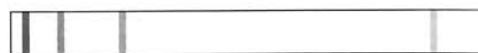
spectrum of light from a hydrogen source in a laboratory on Earth
